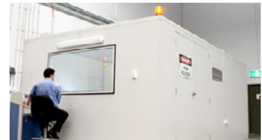
The new Impulse Test Laboratory is capable of simulating lightning strikes and switching surges in accordance to IEC, ANSI/IEEE international standards. The Impulse Voltage generator is rated at 300 kV (15 kJ) and simulates lightning impulse waveform of 1.2/50  $\mu$ s. These in-house facilities provide flexibility to examine and improve existing product design and prove new prototype design concepts which greatly reduces the time and cost of development.
